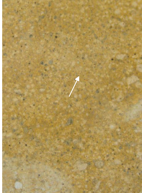
Underside of detached paint flake at 20X
